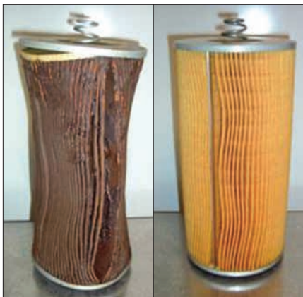
Figure 1: Before and after a collapse test
